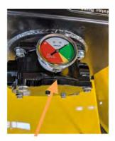
Hydraulic Filter Indicator Gauge – Located on the hydraulic
