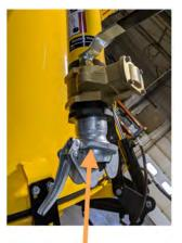
Suction Valve Lever up – Closed Lever down - Open
