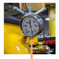
Vacuum Gauge Located on Filter Tank elbow near top of tank
