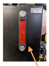
Temperature and Fill Level Gauge. Located on hydraulic tank, curbside
