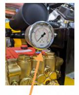
Water Pressure Gauge Located on top of the Giant Water Pump
