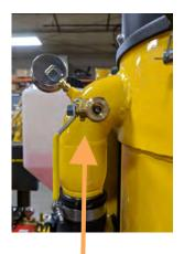
Vacuum Pump Lubrication Valve Located on Air Filter Tank
