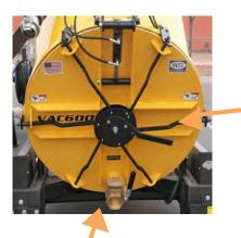
**Rear Door Lever** Lever up – unlatch Lever down - Latch
