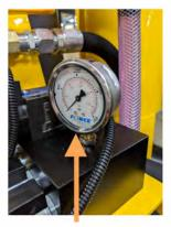
**Hydraulic Pressure Gauge** Located between vacuum silencer and engine.
