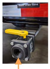
Water System Drain Valve Located curb side forward of axle
