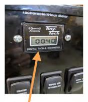
Hour Meter – Located on control panel curbside
