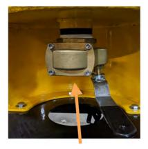
Filter Bag House Drain Valve Lever out – Open Lever in - Closed
