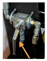
Water Pressure Valve Lever Vertical – Pressure Lever Horizontal – Circulate Located below hose reel
